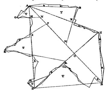
The two main lines which I should recommend to be measured through it are marked A B and C D; A C, C B, B D, D A are the connecting lines. a a a, are the offsets, or perpendicular
